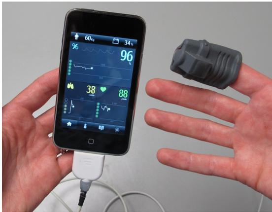
Figure 1: First prototype of the Phone Oximeter
